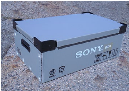
Returnable container used to transport components at Sony Global Manufacturing & Operations Corporation
