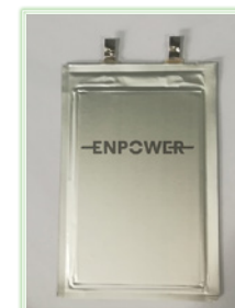
Lithium-ion battery (prototype) jointly developed by SoftBank and Enpower Greentech
