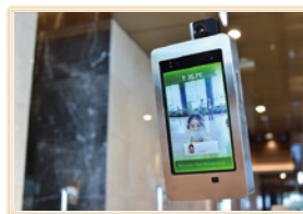
Facial-recognition entry-exit system with a temperature-sensing function
