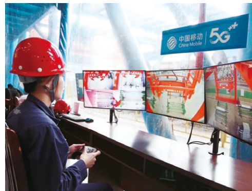
A worker operated a loader with a remote controller in the smart green factory built by Guangxi subsidiary
